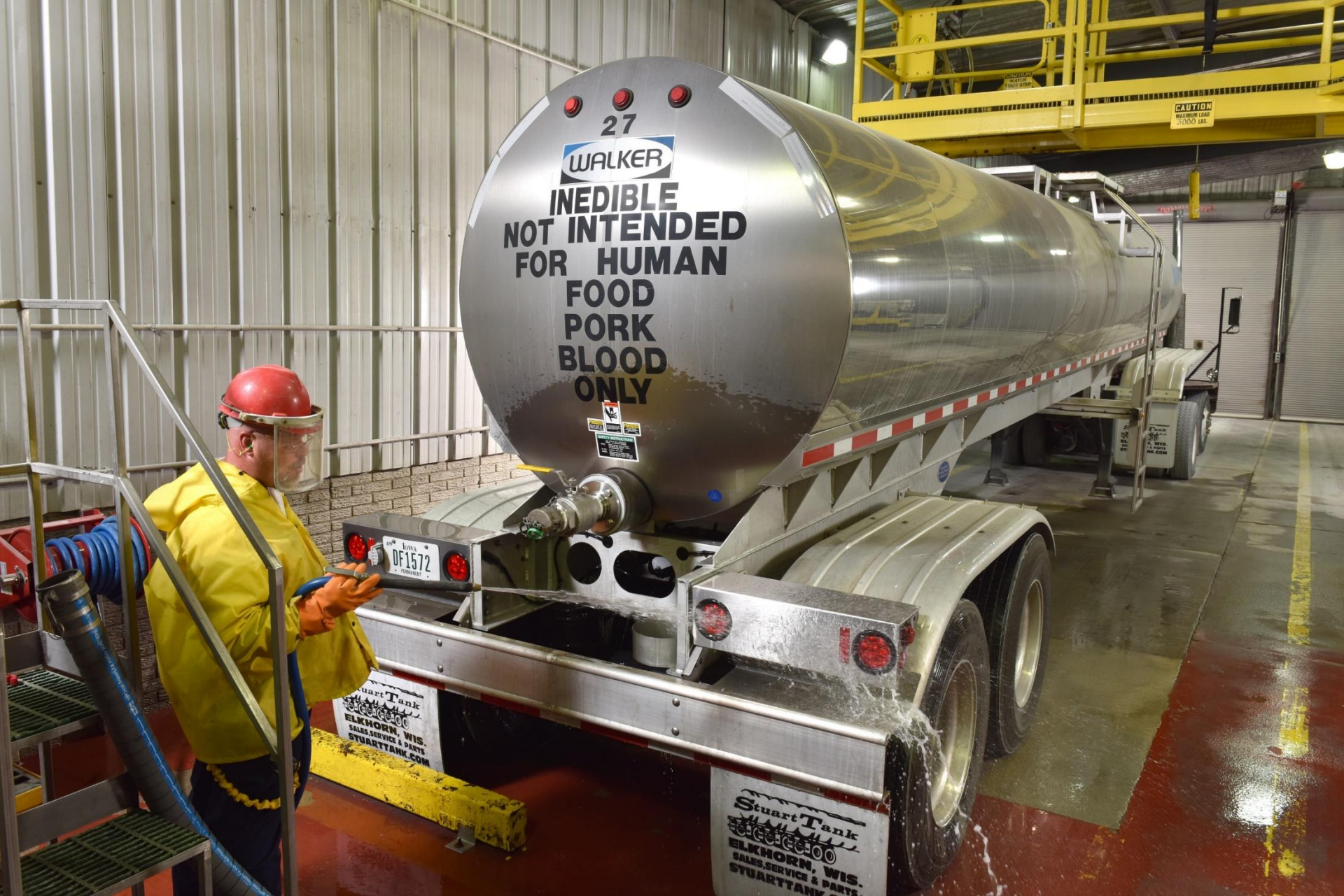
Tankers are sanitized prior to unloading.
