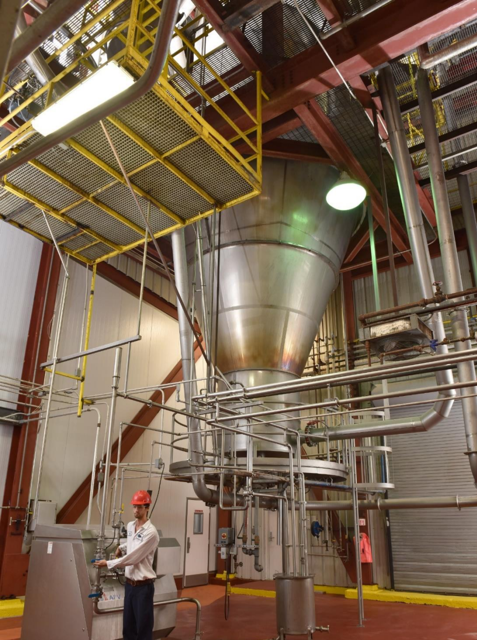
CCP of 80° C minimum outlet air temperature is maintained on dryers and is continuously monitored.
