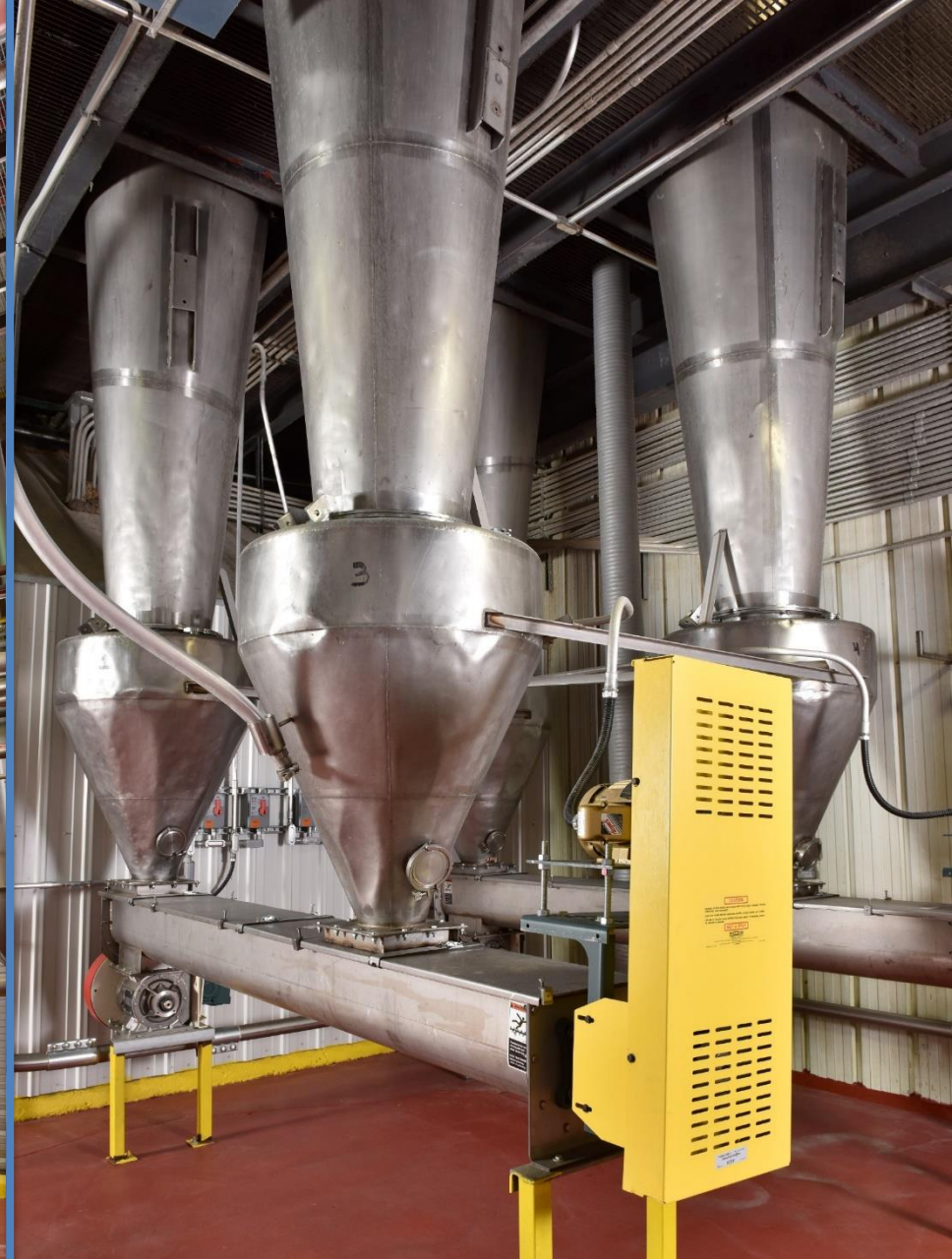
CCP of 80° C minimum outlet air temperature is maintained on dryers and is continuously monitored.
