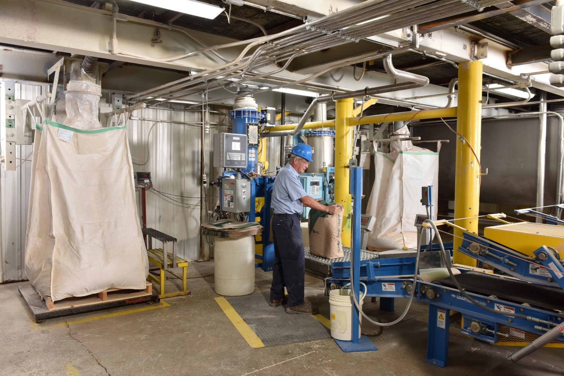
Packaging lines for bagged and bulk product. Note dry side employees wear light blue shirts.
