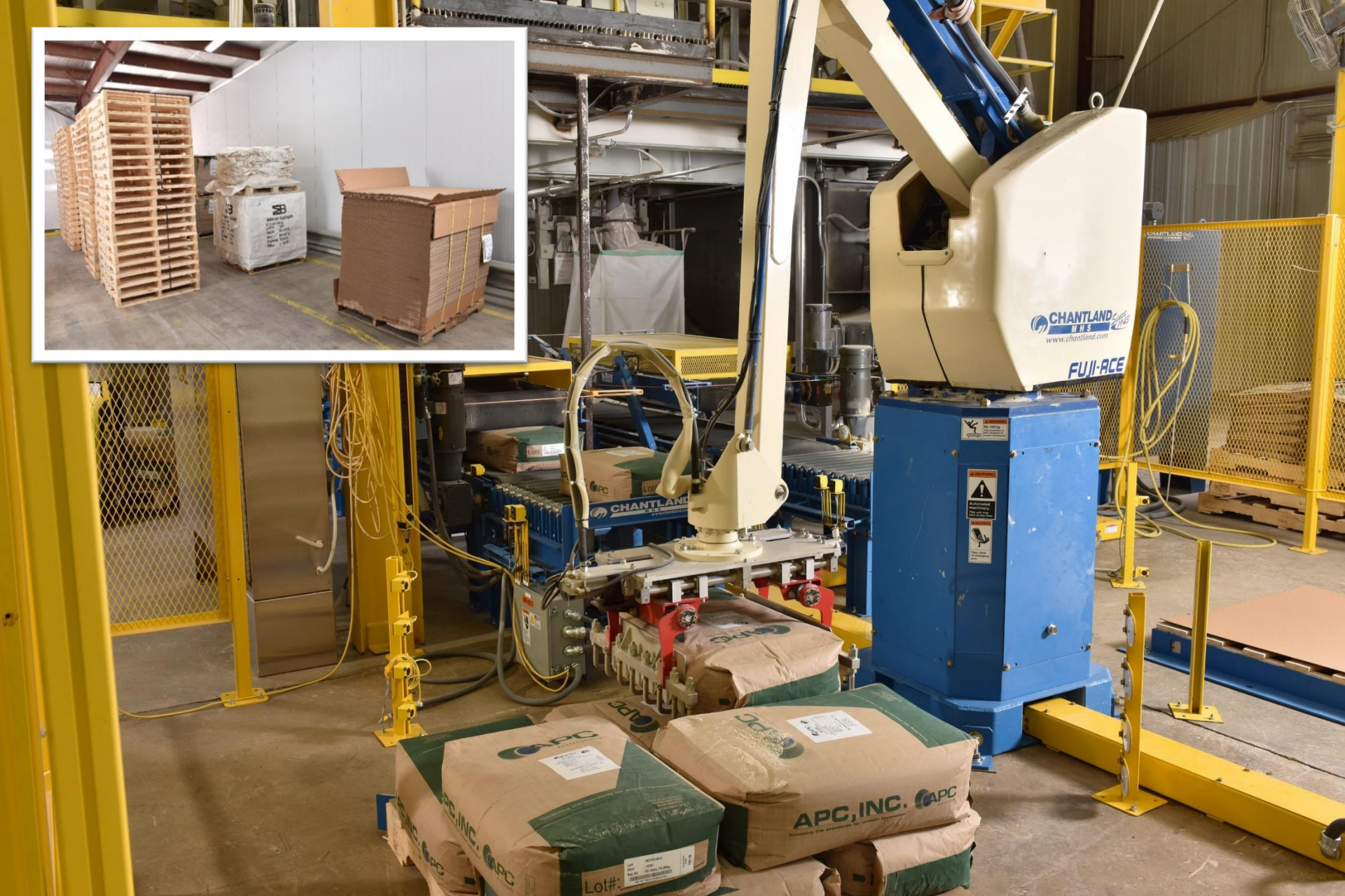
Packaged product is stacked utilizing advanced technology. Only all new packaging materials are used including pallets, totes and bags.
