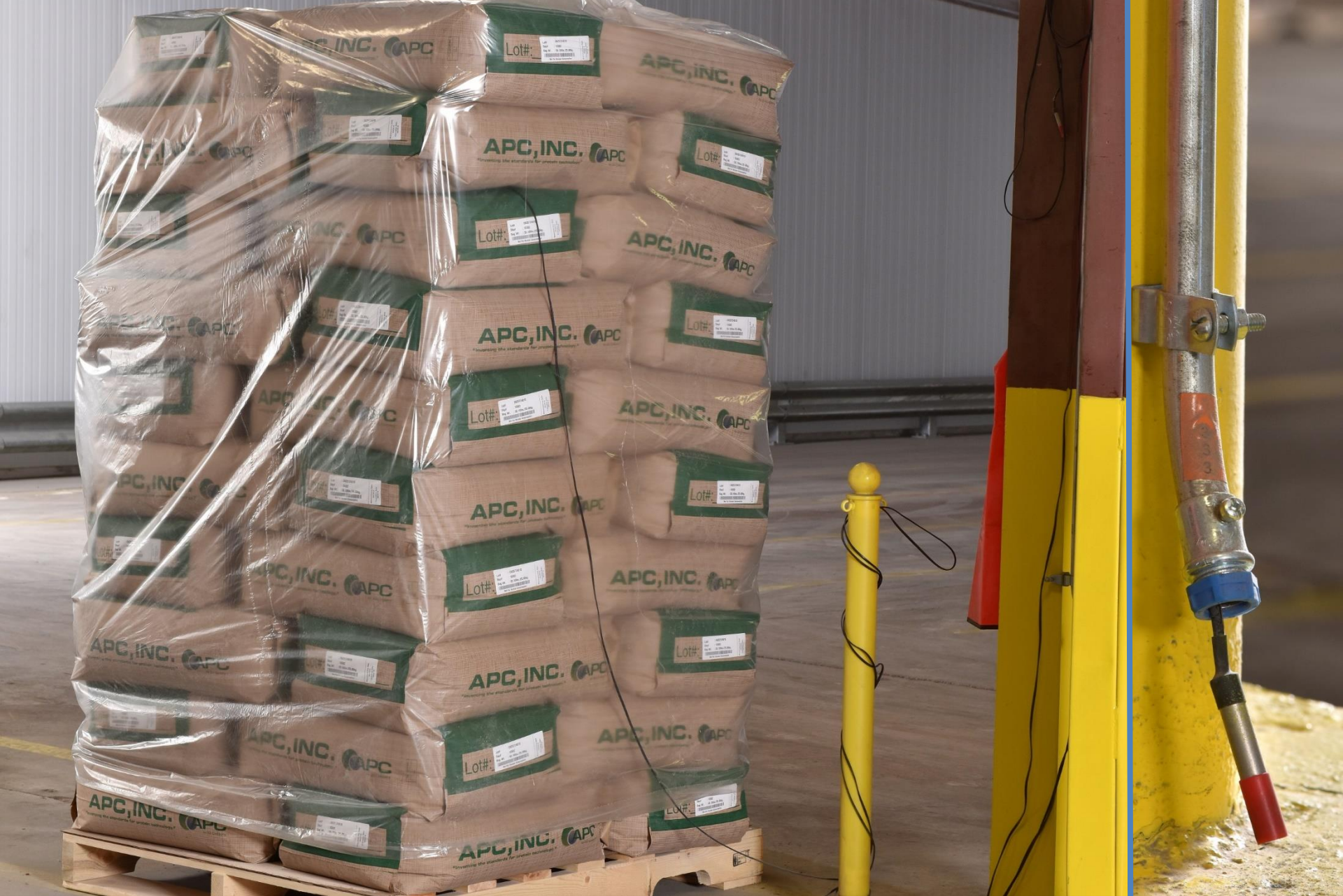
Product is monitored via probes placed in the middle of material with alarms to assure temperature is maintained throughout the holding period.
