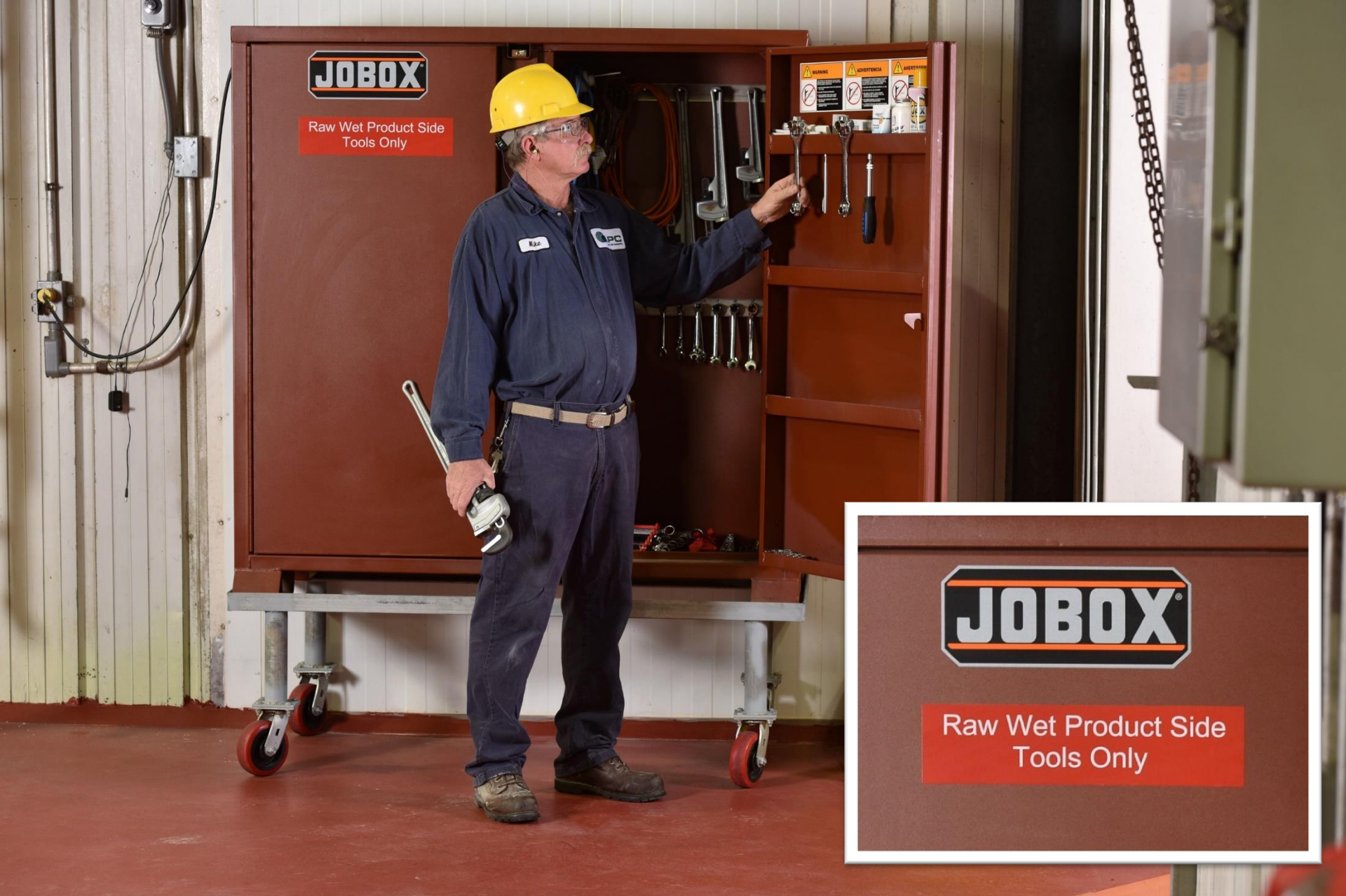
Maintenance workers utilize dedicated wet side or dry side tools. Note maintenance and management employees wear dark blue shirts.
